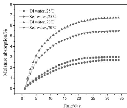
**Fig.1** Moisture absorption with exposure time for sandwich composites
