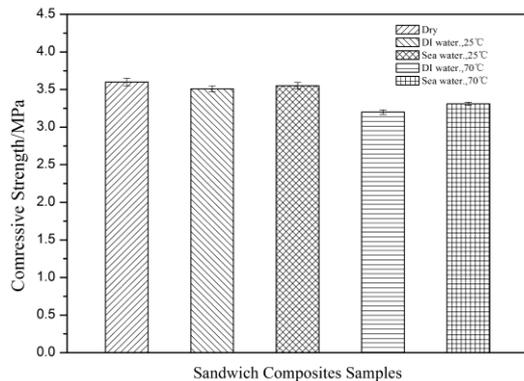
**Fig. 2** The FCS of dry and moisture absorbed specimens
