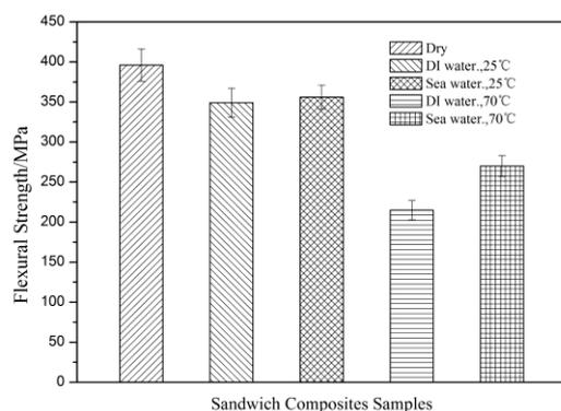
**Fig.5** The flexural strengths of dry and moisture absorbed specimens
