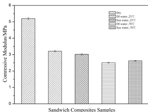
**Fig.3** The compressive modulus of dry and moisture absorbed specimens
